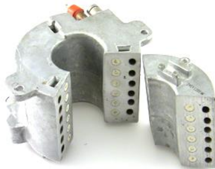
Figure 1.16 Cut view of a single-part thermoblock
