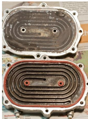
Figure 1.15 Inside a two-part thermoblock
