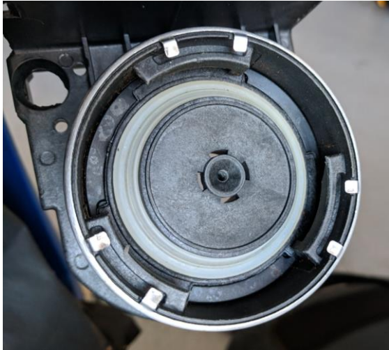
Figure 2.21 Group head attached to the casing
